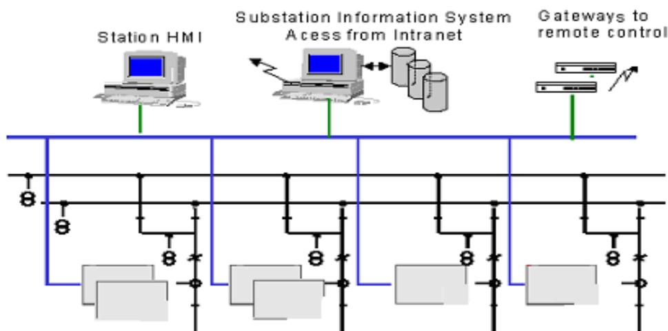
The process bus must be set up so that a malfunction in one bay unit will not cause a breakdown on the rest of the process bus. A bus system must be compatible to products from different manufacturers. A protocol of some sort must be agreed upon by the manufacturers of equipment. The standards IEC 61850-8 for station bus and IEC 61850-9 for process bus, is most likely to be this common platform that manufacturers will agree upon.
