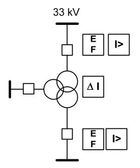
The transformer bay terminal shall contain the following functions:
