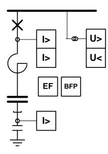
The Capacitor bank bay terminals shall contain the following functions:
