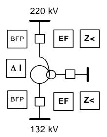
The transformer bay terminals shall contain the following functions:
