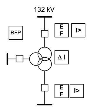
The transformer bay terminal shall contain the following functions:
